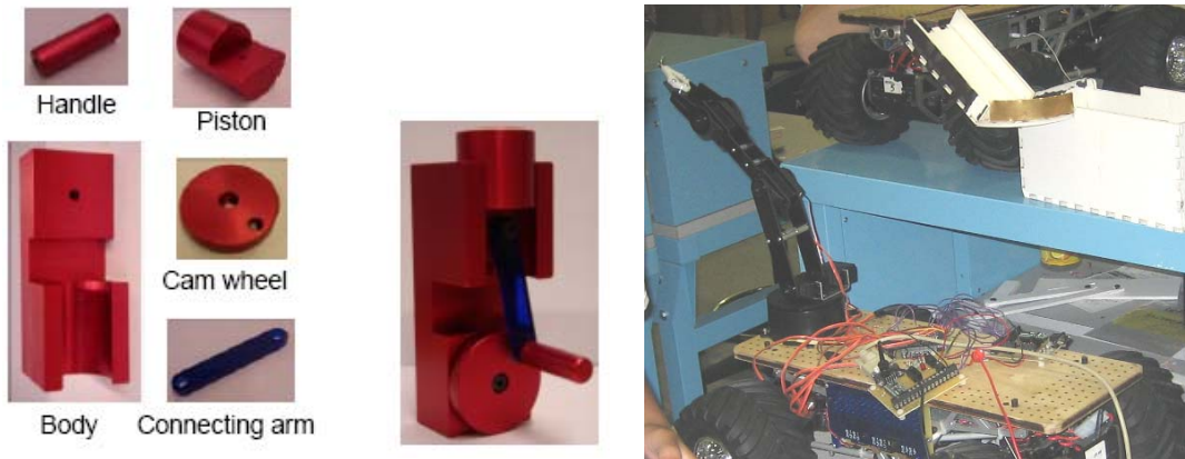
Figure 5: Piston project from years 1 and 2 (l), 4 Degree of freedom arm from year 4 (r)
